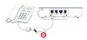
telephone adaptor **(B)** using a multi socket extension if required (not supplied).
